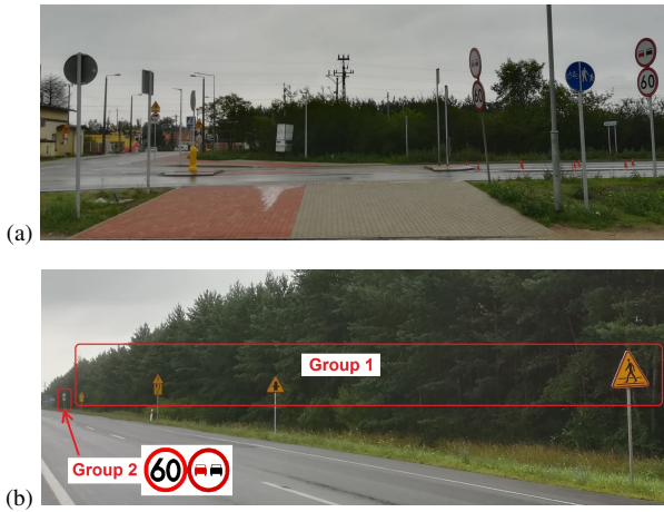
Fig. 2. Compaction of traffic signs in a small area related to different movement directions and possible grouping of them (own source)
