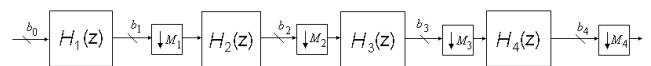
Fig. 1. A typical multistage decimation filter used to remove the quantization noise in the oversampled ADC.
