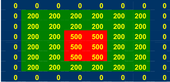
Fig. 8. An example input image A surrounded by zeros used in verification of designed processor. Values are given in [nA]
