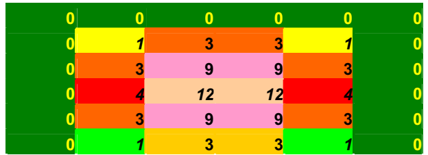
Fig. 12. Output image B after filtration of a normalized image A using the filter mask shown in Fig. 9
