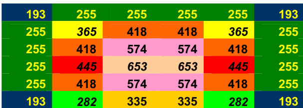
Fig. 10. Output image B after filtration of example image A by the filter mask shown in Fig. 9. Values are given in nA
